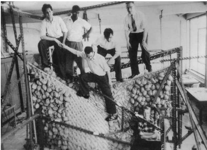
Figure 26 the plywood model severely overloaded.
